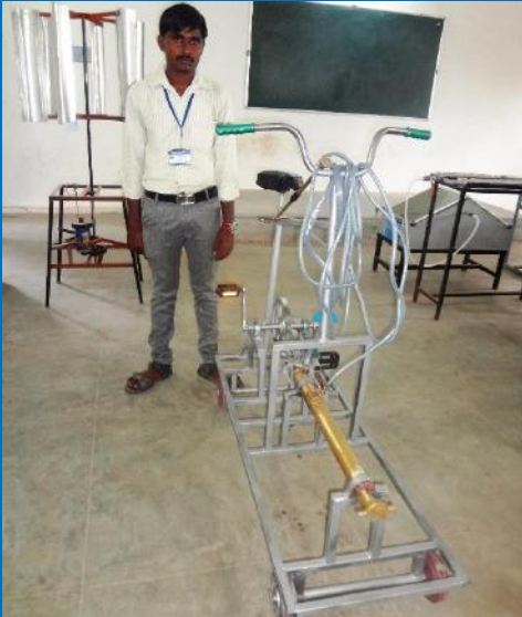
Pedal Operated Agricultural Sprayer
